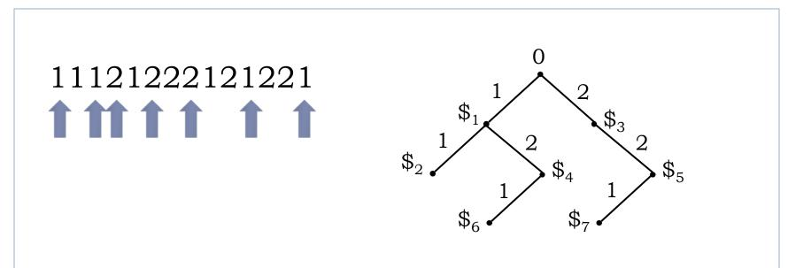
Create a trie while scanning through a string. The compressed string contains pointers to this dictionary.
